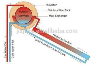
Fig. 2 Flat plate Solar water heater<sup>[2]</sup>
